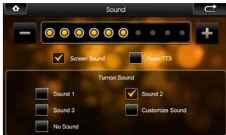
Click “Screen sound” in this interface to enable or disable the sound of screen operations, “Open TTS” is to enable the speech broadcasting function. TTS speech engine gives a clear broadcasting of the function name every time you enter into a function. English and Chinese speeches are supported for the moment. You can listen to the sound by clicking the start-up sound directly; and the general volume can be adjusted by dragging the slide directly. User-defined start-up music
