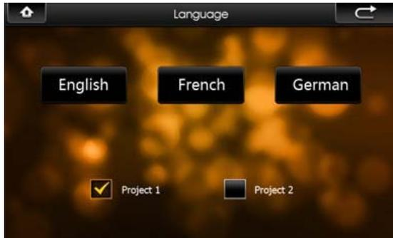
Click the icons of the corresponding language in this interface or choose the interface project, the system will save the setup automatically when the setup is closed, and return to the previous menu. (The system will be required to restart after the interface project is changed.)
