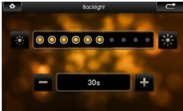
Then, drag the slide block to set. Select No Screen Saver, then the screen saver will be disabled. After setting, close the current window to save.
