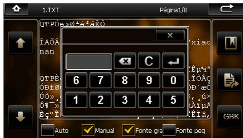
Click the number key on screen to input the page number to jump to, when inputting, click button to backspace for deleting; click button to clear input block, after inputting page number click button to jump to the page of selected number.
